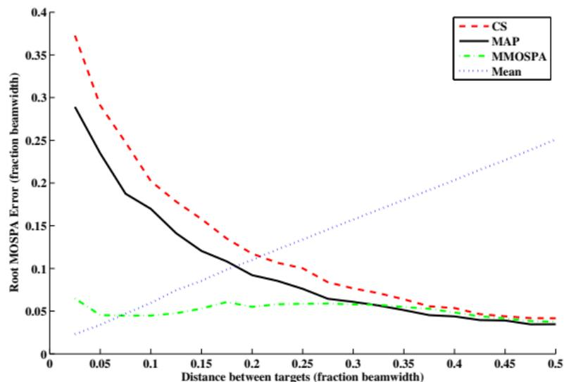
5-element linear array. One target was fixed at the boresight ( $0^\circ$ ) and the other was moved across the array.  $\text{SNR} \approx 20$  dB.
